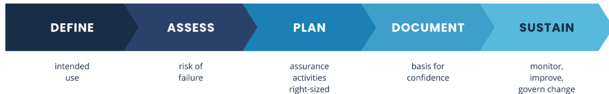
Figure 1. Computer Software Assurance Transition Path
